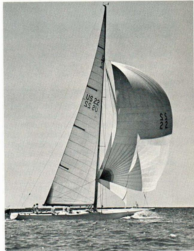
*INTREPID shows how an 80% Staysail should be used - tack aft, minimum interference with spinnaker, clew sheeted to boom for open slot and attached flow with quartering wind.*
