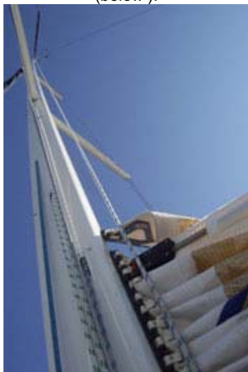
Pre-Bend is measured at point of maximum deflection between S1 and S2 (below).
