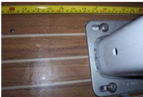
Pre-Bend is measured at point of maximum deflection between S1 and S2 (below).
