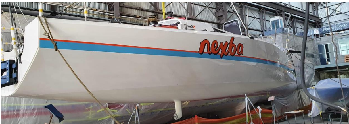
Figure 3 Nexba hull showing sail drive (propeller location) [4]
