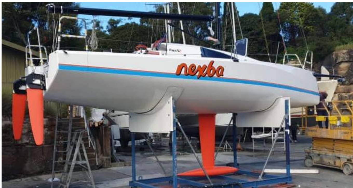
Figure 1 High visibility appendages (rudders and keel) [Source: Skipper]
