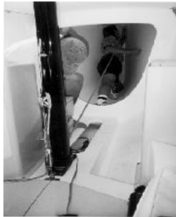
Check the mast butt position
