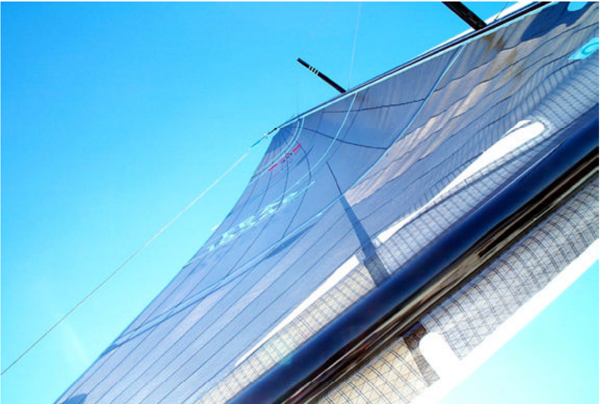
Medium Trim Settings: 11 knots true wind, 50% backstay, outhaul eased 25mm, cunningham tensioned till luff has hint of
