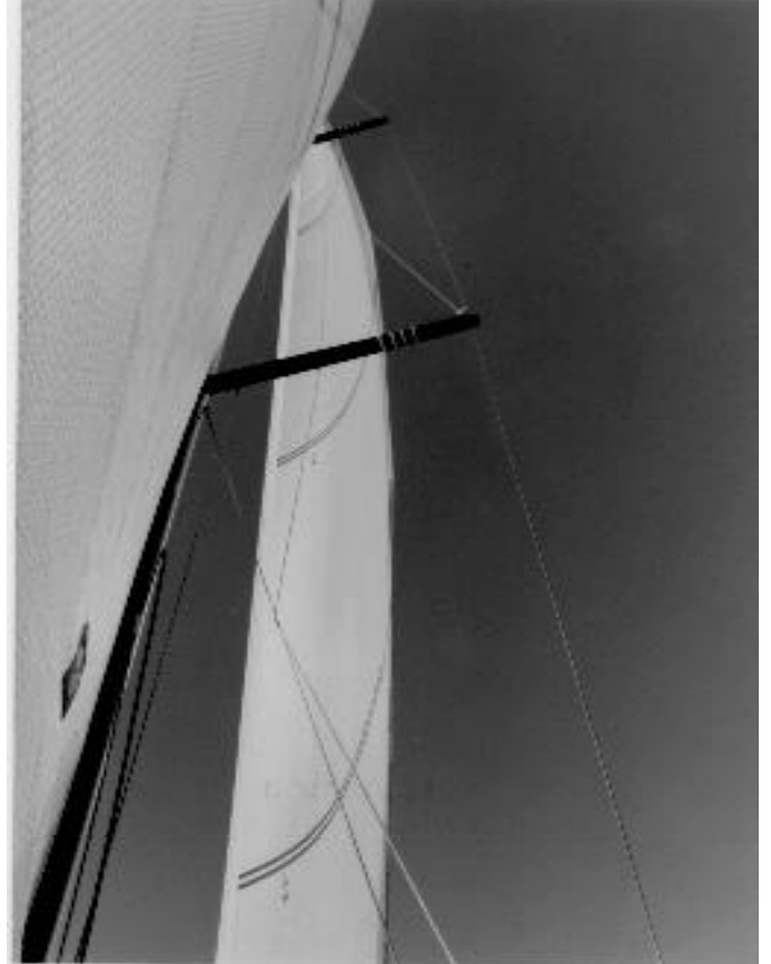
Tight Twist Profile: CODE 2 jib 12 knots true wind trim 375mm (15") at top and bottom spreader, lead at median.
