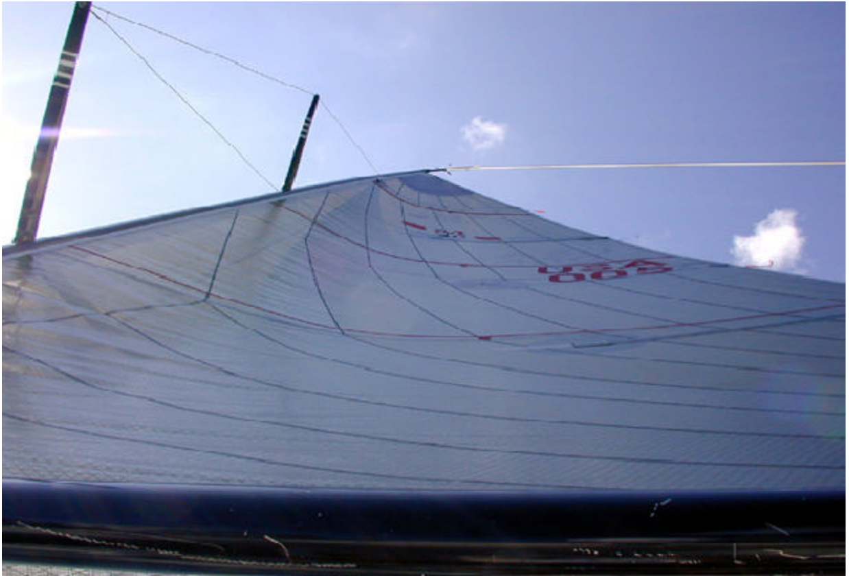
Light Air Trim: 7 knots true wind full power, backstay off, outhaul eased 75mm, cunningham eased allowing hint of horizontal wrinkles, mainsheet eased (top batten 5 degrees to leeward), traveler above centerline.
