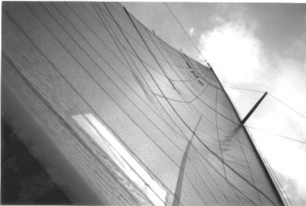
Maximum Depowered: 19 knots true wind, (hanging on with the CODE 2), maximum flattening all controls, sheet eased 150mm from stall to keep the boat on its feet and to allow the driver to bear off for chop without excess heel.
