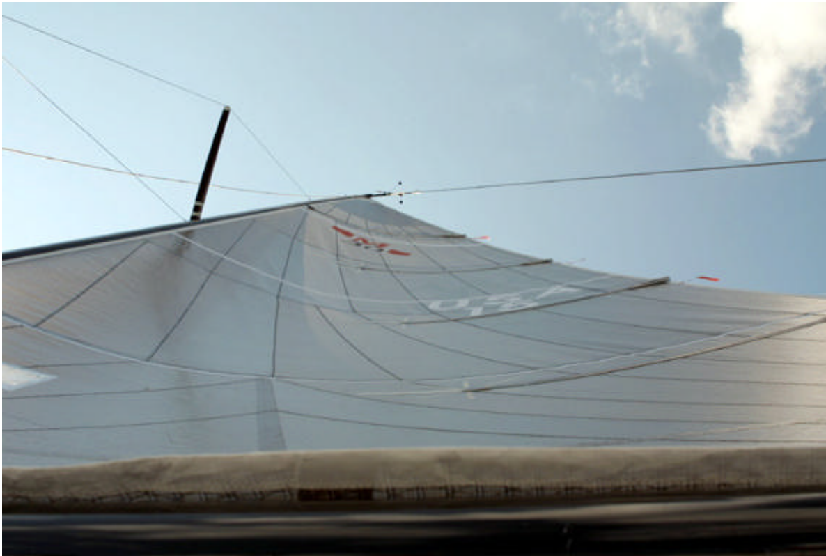
Depowered and Twisted for Speed: 15 knots true wind with 70% backstay, maximum outhaul, sheet eased 125mm from stall.
